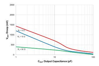
Figure 12. Output Voltage Droop at Switching Over from V<sub>IN1</sub> (5V) to V<sub>IN2</sub> (3.3V)
