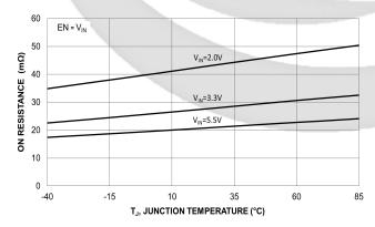
Figure 4. On-Resistance vs. Temperature
