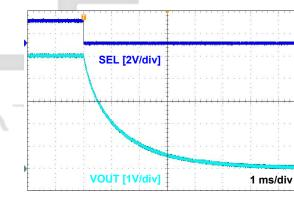
Figure 14. Turn-On Response  $V_{IN1}$ =5.0 V,  $C_{IN}$ = $C_{OUT}$ =10  $\mu$ F,  $R_L$ =150  $\Omega$ , EN=Low
