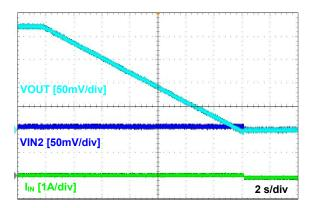
Figure 19. True Reverse Current Blocking Release  $V_{IN1}$  or  $V_{IN2}$ =3.3 V,  $V_{OUT}$ = From 3 V to 3.4 V,  $C_{IN}$ = $C_{OUT}$ =10  $\mu$ F
