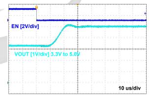
Figure 16.  $V_{\text{OUT}}$  Switchover from 5  $V_{\text{IN}}$  to 3.3  $V_{\text{IN}}$  $V_{IN1}$ =5.0 V,  $V_{IN2}$ =3.3 V,  $C_{IN}$ = $C_{OUT}$ =10  $\mu$ F,  $R_L$ =150  $\Omega$
