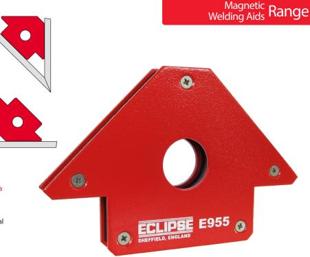
The smaller Heavy Duty Welding Clamps unit is 120mm long and 82mm high with a 14mm width and has a holding force capability of up to 10kg (22lb) pull force rating. The larger Heavy Duty Welding Clamps unit is 160mm long and 102mm high with a 18mm width and has a holding force capability of up to 15kg (33lb) pull force rating. The actual pull force achieved depends on the ferrous material being held (thickness, material type, etc) - the actual pull force achieved is application specific.
