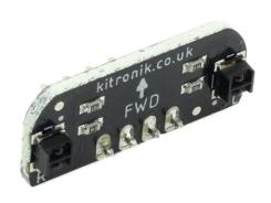
Sensor output: The sensor output voltage changes from the supply voltage to 0V as the sensors pass over light and dark surfaces. Different surfaces will reflect different amounts. A typical light surface will give a value of 0.5V for example. A typical dark surface will give a value of 2.5V (assuming a 3V VCC). The value in a program will depend on the processors ADC range and width.
