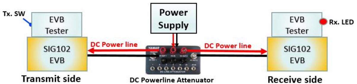
Figure 10 - EVB Tester to EVB Tester
