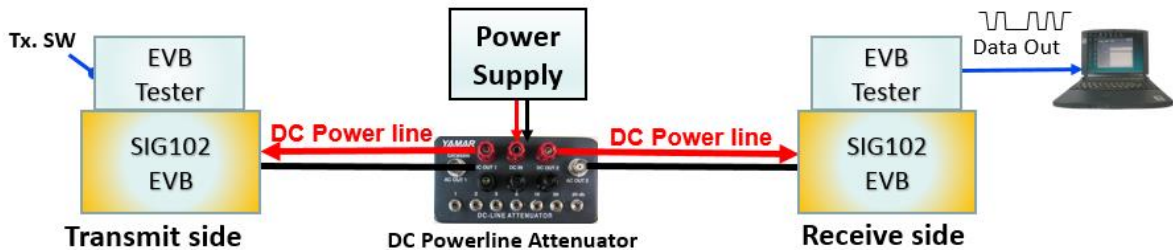
Figure 9 - EVB Tester to PC testing
