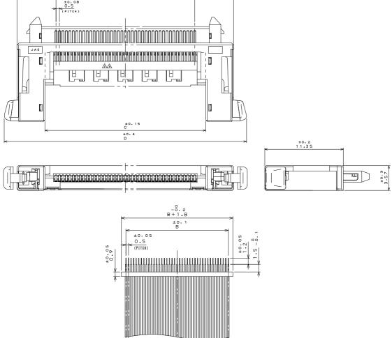
Drawing when cable is connected (for reference)
