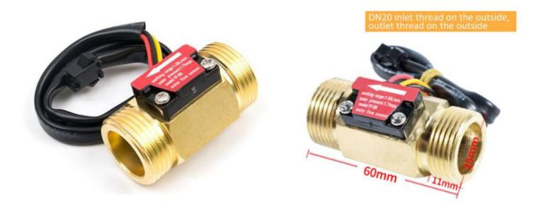
Water flow sensor consists of a copper body, a water rotor, and a hall-effect sensor. When water flows through the rotor, rotor rolls. Its speed changes with different rate of flow. The hall-effect sensor outputs the corresponding pulse signal. This one is suitable to detect flow in water dispenser or coffee machine. Life is longer than plastic body.
