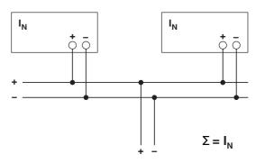
Figure 26 Schematic diagram in parallel operation
