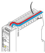
Figure 9 Lay and align connection wiring
