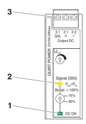
Figure 21 Position of signaling elements
