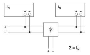
Figure 27 Schematic diagram, redundant operation with diode
