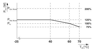
Figure 29 Output power depending on the ambient temperature
