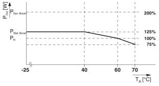
Figure 16 Performance characteristic in static boost
