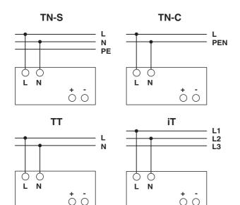
Figure 12 Network configurations in star network
