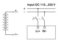
Figure 14 Pin assignment for DC supply voltage
