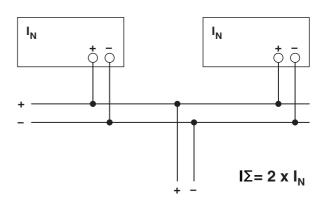
Figure 28 Schematic diagram of increased performance
