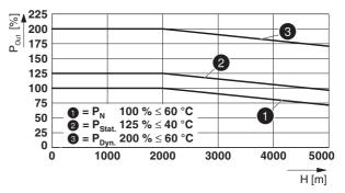
Figure 30 Output power depending on the installation height
