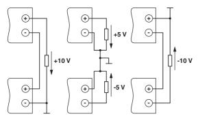
Figure 25 Schematic diagrams in series operation
