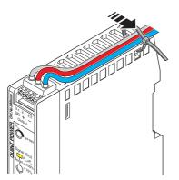
Figure 10 Secure connection wiring with cable binder
