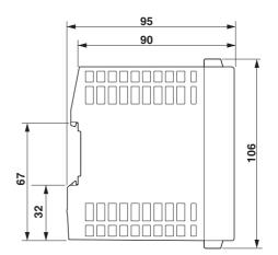
Figure 4 Device dimensions (dimensions in mm)
