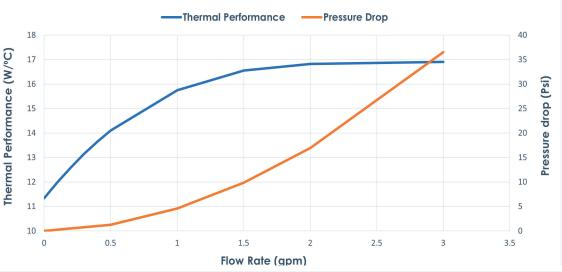
ATS-PHEX-102: Thermal Performance & Pressure Drop vs Flow Rate
