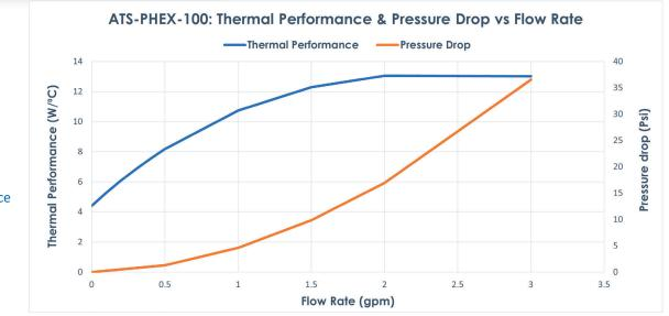
ATS-PHEX-101: Thermal Performance & Pressure Drop vs Flow Rate
