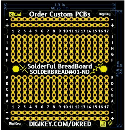
Special Pads for Surface Mount (SMT) 0201 and Up And for Bridge Neighboring Nets at Each End (scrape the mask off first).
