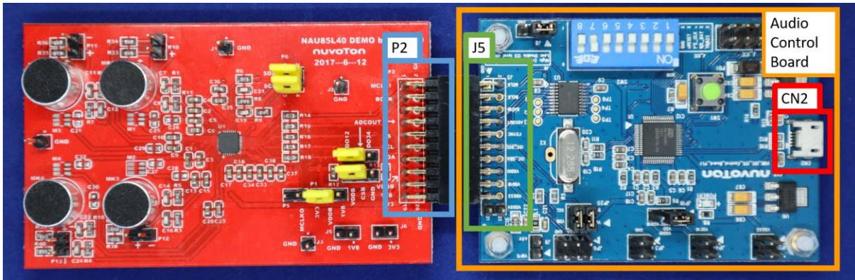
Figure 3-1 Connection Audio Control Board
