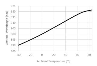
Centroid wavelength versus temperature (T $_{\rm ambient}$  = -40 - 85 °C), 40 A, 100 ns, 0.01% DC
