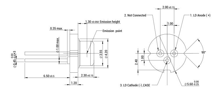
Figure 1: Technical drawing of TO-56 package including dimensions left: side view, right: bottom view, General Tolerance +/- 0.1 mm, Lead finish Au
