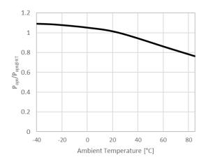
$P/P_{25^{\circ}C}$  versus temperature ( $T_{ambient}$  = -40 - 85 °C), 40 A, 100 ns, 0.01% DC
