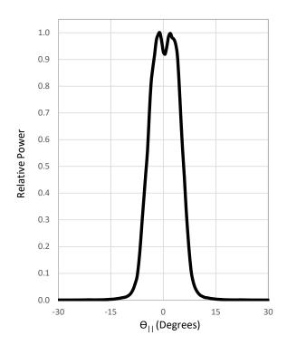
Far-Field parallel to p/n junction, 40 A,  $T_{ambient}$  = 25 °C , 100 ns, 0.01% DC
