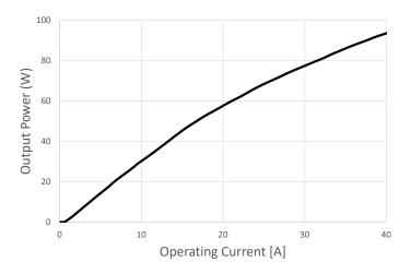
Typical Optical Output Power versus operating current measured at  $T_{\rm ambient}$  = 25 °C, 100 ns, 0.01% DC
