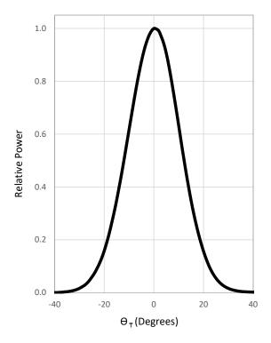
Far-Field perpendicular to p/n junction, 40 A,  $T_{\rm ambient}$  = 25 °C, 100 ns, 0.01% DC
