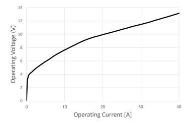
Typical operating voltage versus operating current measured at  $T_{\rm ambient}$  = 25 °C, 100 ns, 0.01% DC
