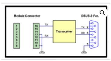
The RS232 module is equipped with a female DSUB9 connector so that the add-on board can be connected to a PC (or a USB to serial adapter) directly or by using a 1:1 male / female cable (this module is a peripheral or DCE).
