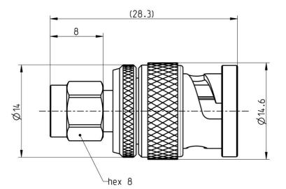
Connector parts Center contact Outer contact SMA side Outer contact BNC side Dielectric Gasket Coupling nut SMA side MaterialPlatingBrassgold platedCuBe or equiv.gold plated NickelBrassPTFESiliconeCuBe or equiv.CuBe or equiv.Gold
