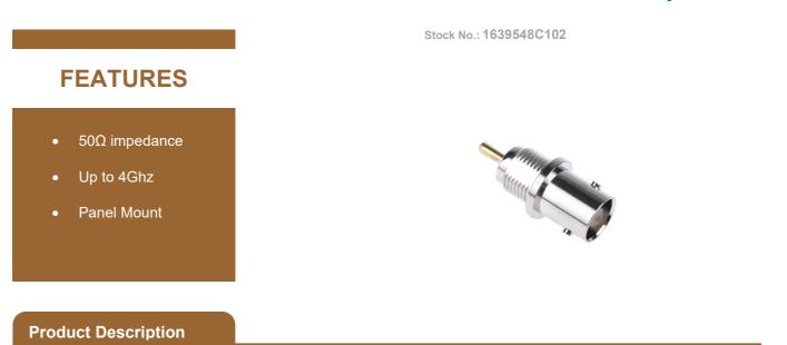
BNC connector is a front mount bulkhead socket connector with a 50  $\Omega$ . With a body plating made from nickel and the male contact made from brass, these BNC connectors are made for brilliant quality. They will terminate to popular RG coax cables using a 4GHz frequency. This BNC connector is a female gender.
