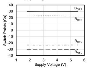
Figure 7. Switch points versus supply voltage (T<sub>A</sub>=25°C)
