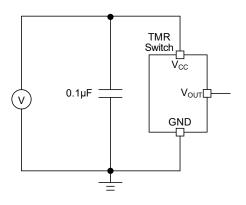
Figure 15. Application circuit diagram
