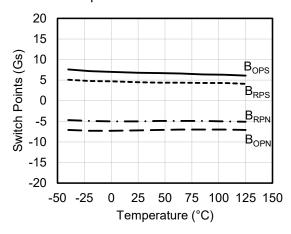
Figure 14. Switch points versus temperature ( $V_{CC} = 3 \text{ V}$ )
