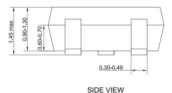
Figure 17. Package outline of SOT23-3 (unit: mm)
