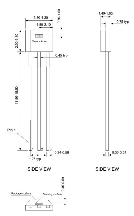
Figure 18. Package outline of TO92S (unit: mm)
