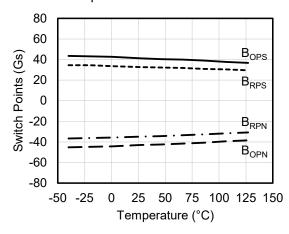
Figure 13. Switch points versus temperature ( $V_{CC} = 3 \text{ V}$ )
