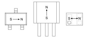
Figure 2. Sensing direction
