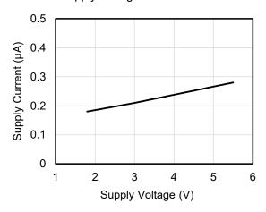
Figure 5. Supply current versus supply voltage (T<sub>A</sub>=25°C)
