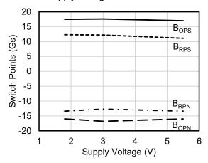
Figure 6. Switch points versus supply voltage  $(T_A=25^{\circ}C)$
