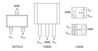
Figure 4. Pin configuration
