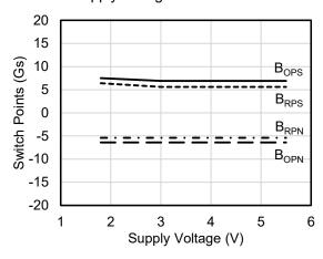
Figure 9. Switch points versus supply voltage (T<sub>A</sub>=25°C)
