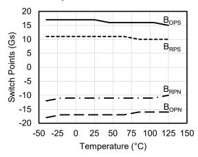
Figure 11. Switch points versus temperature ( $V_{CC} = 3 \text{ V}$ )
