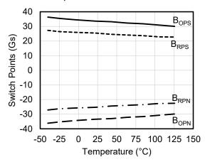
Figure 12. Switch points versus temperature ( $V_{CC} = 3 \text{ V}$ )
