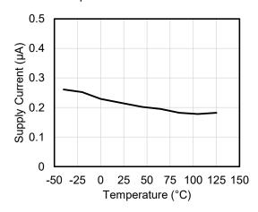
Figure 10. Supply current versus temperature ( $V_{CC} = 3 \text{ V}$ )
