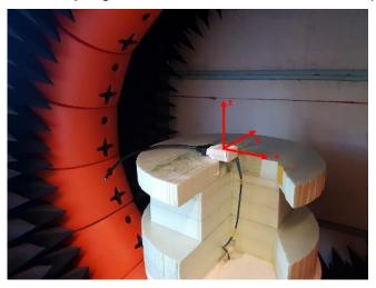
Figure 3. Radiation Pattern Measurement Set-Up
