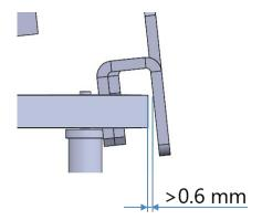
Figure 6 Antenna mounting on main PCB
