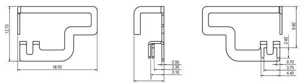
Figure 2. 3D View of the antenna with dimensions (mm)
