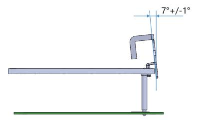
Figure 5. Antenna mounting on main PCB
