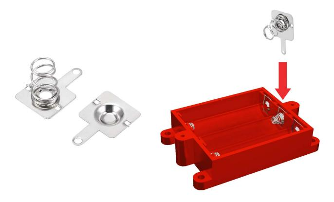
These battery contacts will fit all XYMTEC 3D printable AAA battery compartments. Press the contacts fully into the available slots in the printed part. The solder tabs will extend out the bottom of the part.
