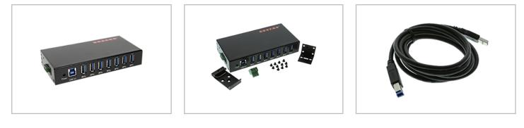
The GM-HU37 Hub is a USB 3.0 specification compliant with up to 5Gbps data transfer speeds depending systems usage. The hub construction is industrial-grade metal with two available mounting options (1) DIN-Rail mount secured to the back panel of the hub and (2) Mounting brackets on either end of the hub secured by 4 screws for each bracket.
