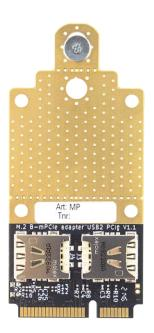
Three adapter variants available routing different data interfaces between host miniPCle socket to the M.2 key B cellular module. USB2/USB3, USB2/PCle x1 or USB2 (only). Chose variant based on support by your host board and cellular module.
