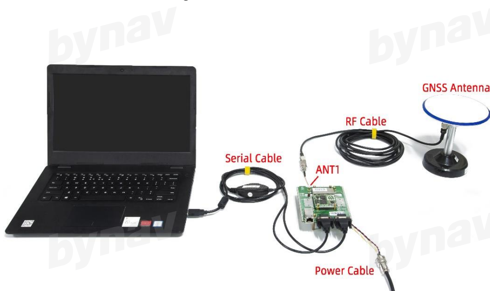
Figure15 Dev board connection
