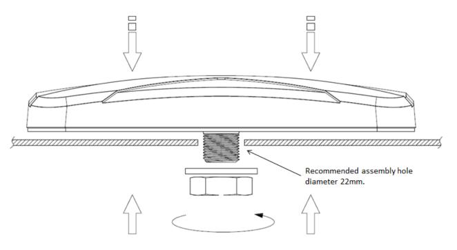
Recommended toque for mounting is 29.4 N,m or 300 kgf,cm Maximun toque for mounting is 39.2 N,m or 400 kgf,cm
