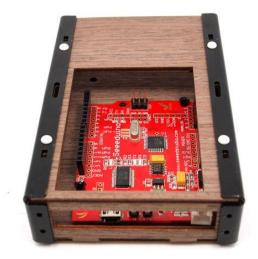
Aluminum bars and Acrylic boards. One Skeleton is a unit that fits Arduino uno/mega, Seeeduino series and 2.8' TFT touch screen. Feel free to stack them up vertically or horizontally with rivets.
