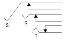
SWITCH CONTACTS OPEN WHEN PLUG IS INSERTED, CLOSE WHEN PLUG IS WITHDRAWN.
