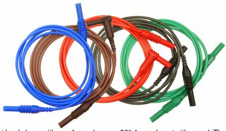
These single test leads have either a 4mm plug or a 90° 4mm plug at either end. The cable is silicone and the total length is 1.5m. Plugs are rated 10A. 1KV CAT III
