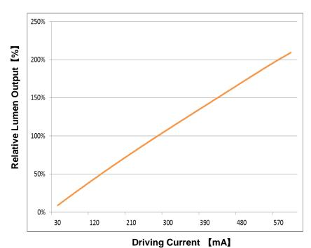
$\bullet$  Scale ratio curve for related efficacy VS driving current,  $T_c$  = 25  $^{\circ}$ C
