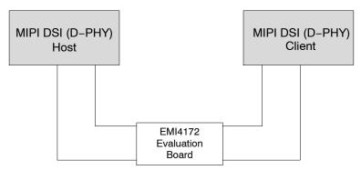
Figure 4. MIPI D-PHY LP Mode Test Setup
