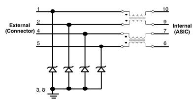
Figure 1. EMI4172 Electrical Schematic
