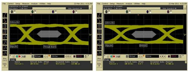
Figure 7. EMI4172 Measured Eye Diagram @ 3.4Gbps (EVB through on left, EVB with EMI4172 on right)
