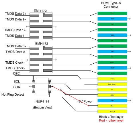
Figure 15. EMI4172 HDMI Type – A Connector Application Diagram
