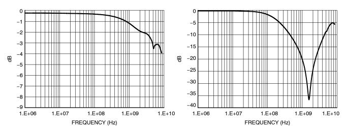
Figure 2. Differential Mode Attenuation vs. Frequency
