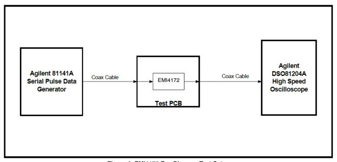
Figure 6. EMI4172 Eye Diagram Test Setup
