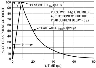
Figure 12. 8 x 20 µs Pulse Waveform
