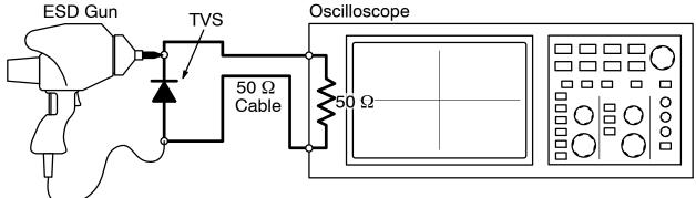
Figure 11. Diagram of ESD Test Setup
