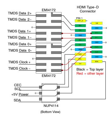
Figure 16. EMI4172 HDMI Type – D Connector Application Diagram
