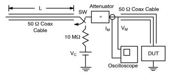
Figure 8. Simplified Schematic of a Typical TLP System
