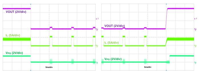
Figure 11. Output Short Protection with PG, IOUT = 4A
