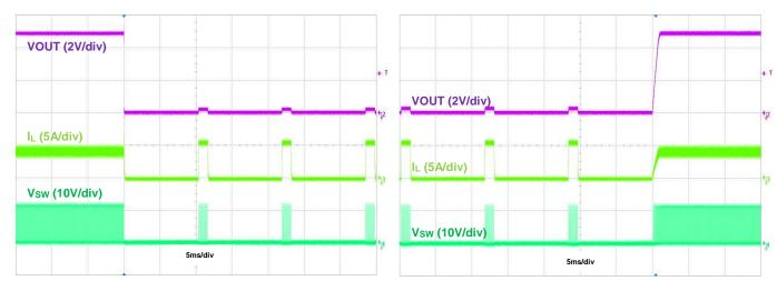
Figure 9. Output Short Protection, IOUT = 4A
