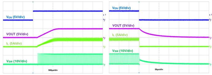
Figure 7. Startup Using EN, IOUT = 4A
