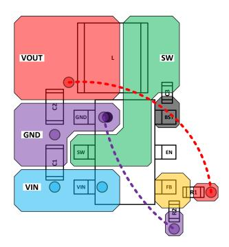
Figure 39. Recommended PCB Layout, TSOT26 Package
