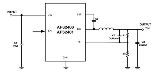
Figure 1. Typical TSOT26 Package Application Circuit
