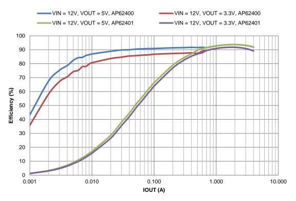
Figure 2. Efficiency vs. Output Current, AP62400 & AP62401
