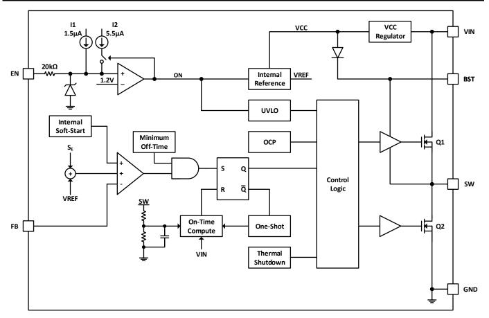
Figure 3. Functional Block Diagram, 6-Pin AP62400/AP62401
