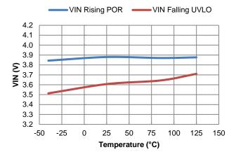
Figure 6. VIN Power-On Reset & UVLO vs. Temperature
