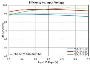
Figure 4 Efficiency versus Input Voltage (ultra-sonic enable)
