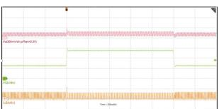
VIN=2.5V to 5.5V, PFM, T<sub>A</sub>=25°C, V<sub>O</sub>=3.3V, I<sub>O</sub>=200mA
