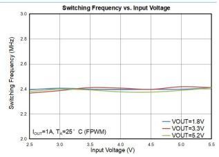
Figure 24. Switching Frequency versus Input Voltage
