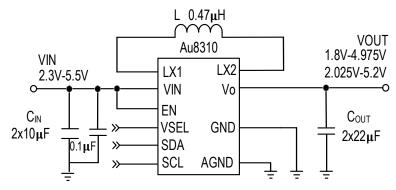
**Figure 41 Typical Application Circuit**
