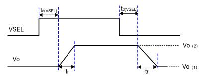
Figure 31 DVS Timing Diagram Using the VSEL Pin
