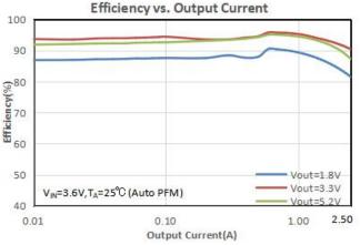
Figure 3 Efficiency versus Output Current (ultra-sonic enable)
