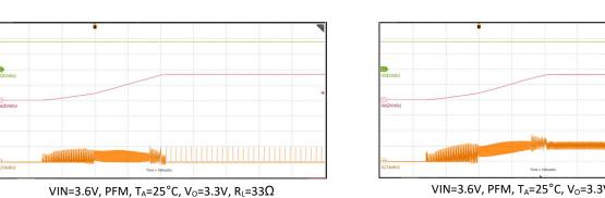
Figure 19 Start-Up waveforms (Light load)
