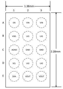
Figure 2 15-Pin WLCSP Package Top View
