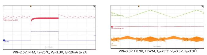
Figure 17 Load Transient Response (Boost)
