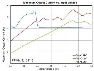
Figure 26. Maximum Output Current versus Input Voltage
