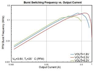
Figure 25. Burst Switching Frequency versus Output Current
