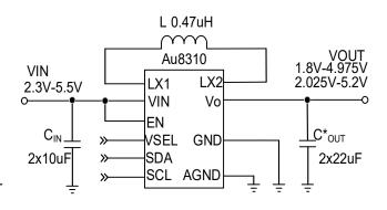
Figure 1 Simplified Schematic
