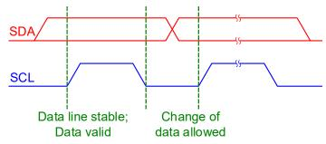
Figure 36 Bit Transfer on the Serial Interface
