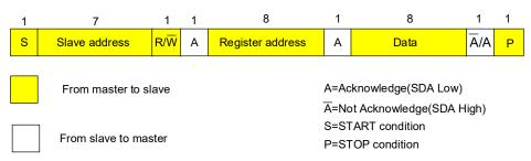
Figure 39 Write Data Transfer Format in Standard, Fast and Fast-Plus Modes
