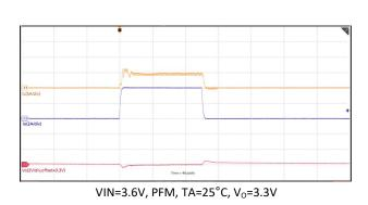
Figure 23. Overcurrent Protection
