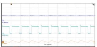
VIN=2.5V, FPWM,  $T_A$ =25°C,  $V_O$ =3.3V,  $I_O$ =100mA
