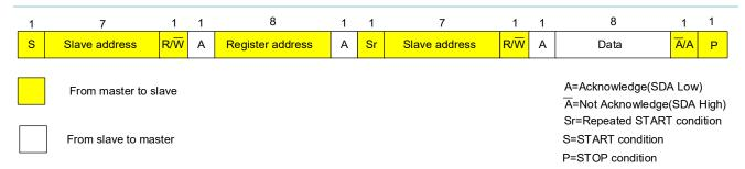
Figure 40 Read Data Transfer Format in Standard, Fast and Fast-Plus Modes
