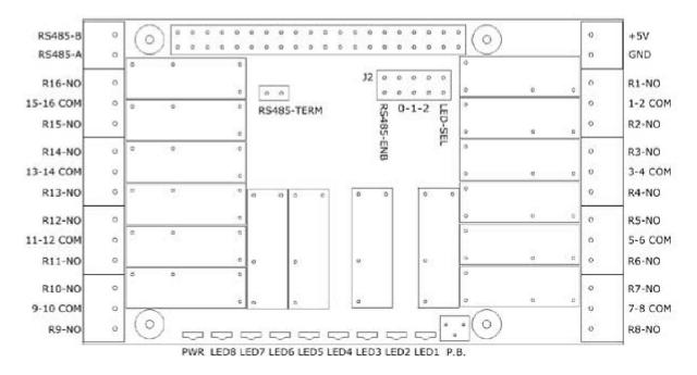
Your 16-RELAYS card comes with appropriate mounting hardware. Up to eight 16-RELAYS cards can be stacked on top of one Raspberry Pi. Eight LEDs indicate the status of their respective relay. An LED is lit when the corresponding relay is energized. The General Purpose Pushbutton GPB is connected to pin 37 of the Raspberry Pi GPIO connector (GPIO26). In order to use the pushbutton you need to write a shell script to accomplish the desired function.
