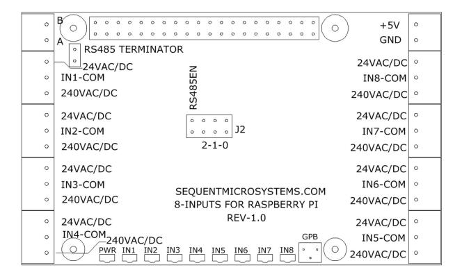
The 8-INPUTS card comes with appropriate mounting hardware. Up to eight cards can be stacked on top of one Raspberry Pi.
