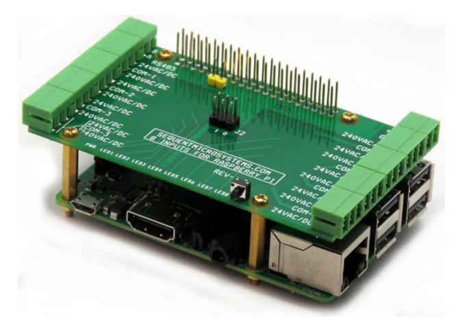
The 8-INPUTS card is a stackable expansion card for Raspberry Pi. It is compatible with all Raspberry Pi versions from Zero to 4. It offers a compact and inexpensive solution for adding up to 64 universal inputs to your Raspberry Pi project. Optically isolated inputs can process signals from 3V to 24V, or from 120V to 240V, AC or DC.
