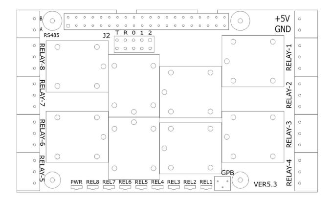
Your 8-RELAYS card comes with appropriate mounting hardware. Up to eight 8-RELAYS cards can be stacked on top of one Raspberry Pi. Eight LEDs indicate the status of their respective relay. An LED is lit when the corresponding relay is energized. The General Purpose Pushbutton GPB is connected to pin 37 of the Raspberry Pi GPIO connector (GPIO26). In order to use the pushbutton you need to write a shell script to accomplish the desired function.
