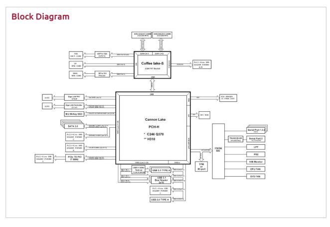
4 ports USB 2.0 through backplane 2 ports USB 3.0 through I/O bracket
