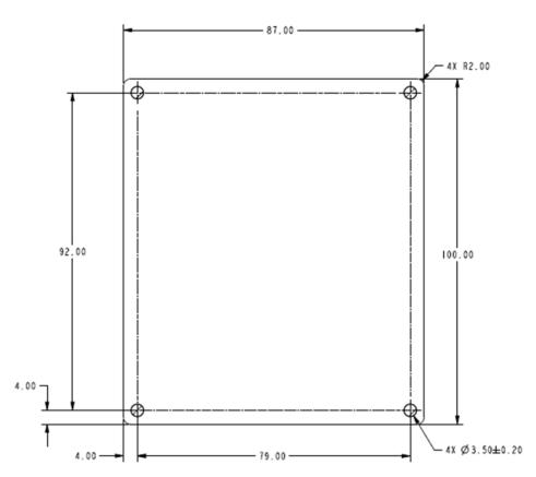
Figure 7-2. Module Mechanical Drawing - Top View
