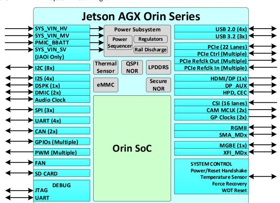
Figure 2-1. System Block Diagram
