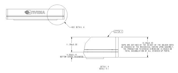
Figure 7-4. Module Mechanical Drawing - Midpoint of the Connector View
