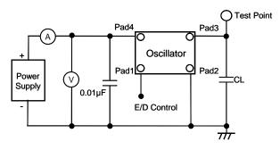
Note: CL includes probe and test fixture capacitance
