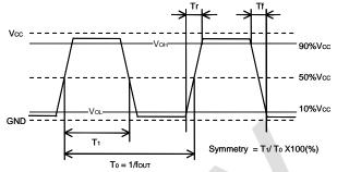
Fig.2 Clock Timing Chart (C-MOS Output)
