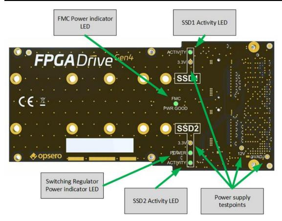
The main components on the bottom-side of the mezzanine card are:
