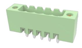
PCB connector Rated current: 8 A Rated voltage: 300 V Pitch: 3.81 mm Mounting: Wave soldering
