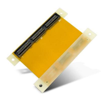
HSMC Flex Cable is equipped with two 160-pin HSMC connectors, one male and female each. It allows user to connect 2 HSMC-interfaced boards together. For example, a Cyclone III Starter Kit is connected to NEEK Upgrade Kit in a brick form by this cable as shown in the pictures below.
