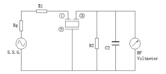
R1+Rg =R2=330 $\Omega$ ±5%,Rg=50 $\Omega$ ; C2=10 PF (Including stray capacitance and capacitance of RF Voltmeter)
