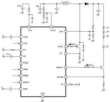
Figure 16. The basic application circuit example
