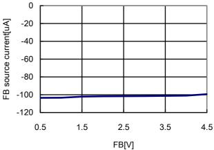
Figure 9. FB source current vs FB voltage
