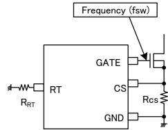
Figure 25. RT pin setting example
