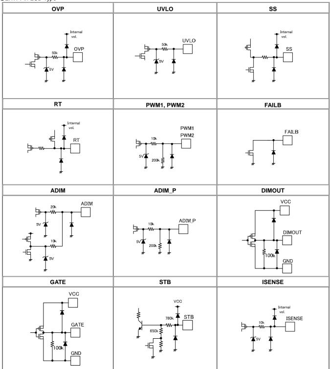
Figure 4-1. Internal equivalent circuit
