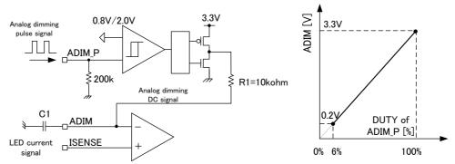
Figure 12. Analog dimming function and character
