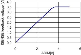
Figure 10. ISENSE feedback voltage vs ADIM
