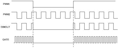
Figure 11. PWM pin function
