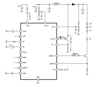
Figure 2. Typical application circuit
