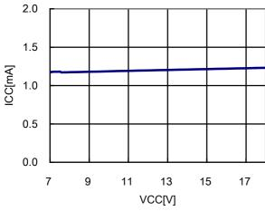
Figure 6. Operating current (ICC) vs VCC
