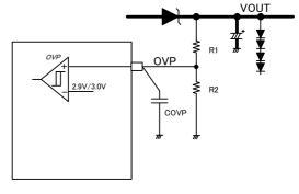
Figure 27. OVP setting example
