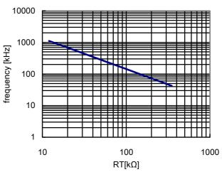
Figure 7. GATE frequency vs RT
