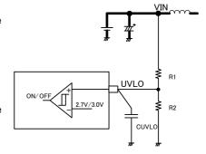
$$VIN_{CAN} = 3.0V \times \frac{(R1[k\Omega] + R2[k\Omega])}{R2[k\Omega]} \quad [V]$$
