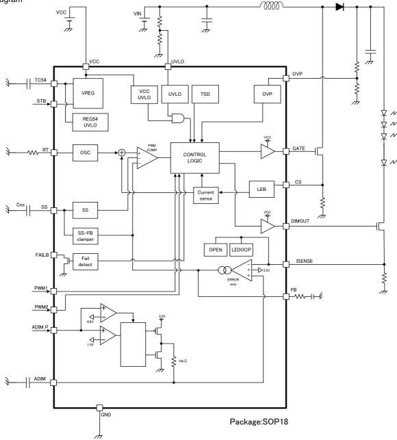
Figure 5. Block diagram
