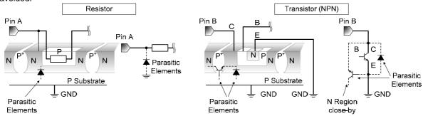
Figure xx. Example of monolithic IC structure
