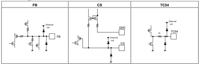
Figure 4-2. Internal equivalent circuit
