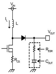
Output capacitor needs to be selected in consideration of equivalent series resistance required to even the stable area of output voltage or ripple voltage. Be aware that set LED current may not be flown due to decrease in LED terminal voltage if output ripple componet is high.
