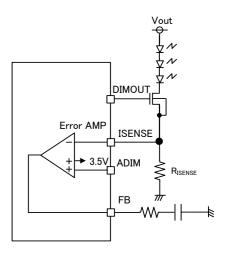
Figure 24. the example of LED current setting
