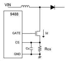
Figure 15. CS pin circuit
