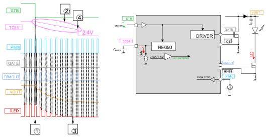
Figure 23. the shutdown waveform and circuit
