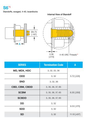
\*1 Printed board mounting hole to be Ø3.12±0.08 [.123±.003] for use with boardlocks.
