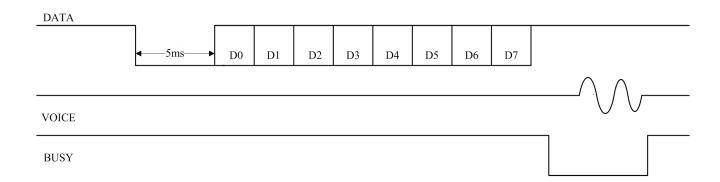
Pull data line low to 5ms(the time range is 5ms-20ms), then send 8-bit data, low bit first, then high bit. Use the ratio of high level and low level to represent the value of each data bit.
