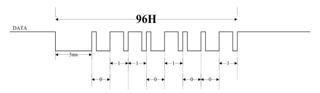
If we want the chip to play the voice content of address 01/02/03/04 in sequence. That is, the code-linking command playback, F3+01+F3+02+F3+03+F3+04. The corresponding sequence diagram can be shown as
