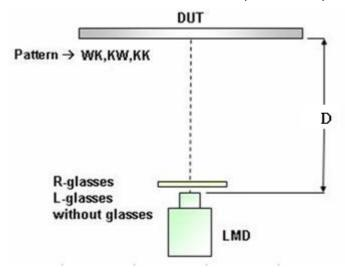
$$Crosstalk_R = \frac{R_L(W, K) - R_L(K, K)}{R_L(K, W) - R_L(K, K)} \times 100\%$$
