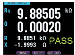
ENLARGE Display Enlarge Measurement Results and Include PASS/FAIL Judgment
