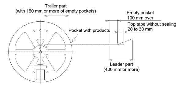
Fig. 13 Taping specification
