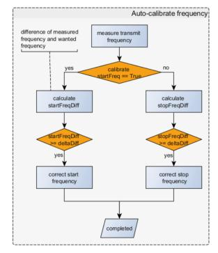
In the first step the transmit frequency of SMR module is measured. a) Afterwards the difference between the target transmit frequency and the measured transmit frequency is calculated. Based on this difference the transmit frequency is changed accordingly and tested again.
