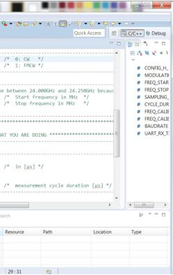
The radar setting can be changed by modifying the parameters in this "CONFIG.h" C) file. For example changing radar configuration to FMCW mode by setting "#define MODULATION (1) "
