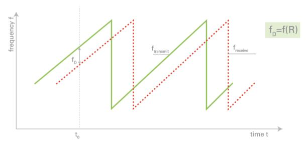
Time-dependent shape of transmit and receive signal of a FMCW radar with sawtooth modulation scheme
