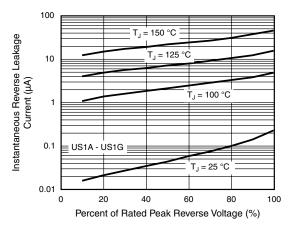
Figure 4. Typical Reverse Leakage Characteristics
