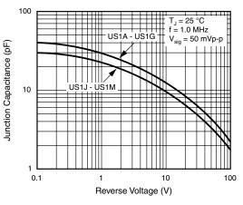
Figure 7. Typical Junction Capacitance
