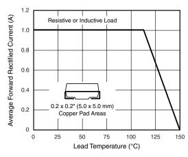
Figure 1. Forward Current Derating Curve
