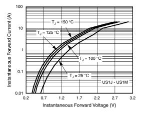
Figure 5. Typical Instantaneous Forward Characteristics
