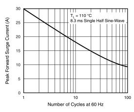
Figure 2. Maximum Non-Repetitive Peak Forward Surge Current
