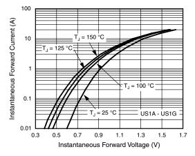
Figure 3. Typical Instantaneous Forward Characteristics
