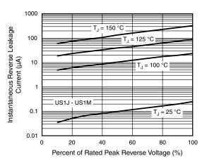
Figure 6. Typical Reverse Leakage Characteristics
