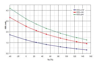
11.6.  $I_{DD}$  vs.  $V_{DD}$
