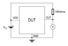
Note 1 -  $B_{\text{OP}}$  is determined by putting the device under magnetic field swept from  $B_{\text{RPmin}}$  up to  $B_{\text{OPmax}}$  until the output is switched on.
