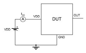
Note 1 - The supply current I<sub>DD</sub> represents the static supply current. OUT is left open during measurement.
