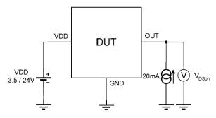
Note 1 - The output saturation voltage  $\rm V_{DSon}$  is measured at  $\rm V_{DD}$  = 3.5V and  $\rm V_{DD}$  = 24V.
