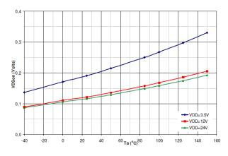
11.4.  $V_{DSON}$  vs.  $V_{DD}$
