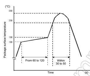
Fig. 13.1.1 An example of a temperature profile when lead(Pb)-free solder is used
