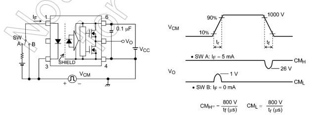
Fig. 12.1.8 Common-Mode Transient Immunity and Waveform
