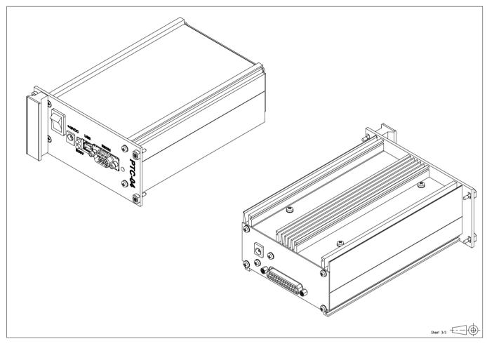
Figure 21-2: Mechanical 3D View
