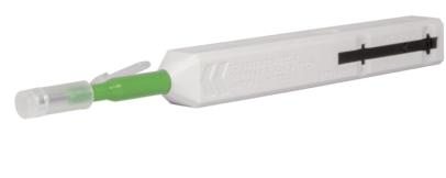
The *Fiber Optic Pen Cleaner for SC/ST/FC Ferrules* is an innovative design of the traditional fiber end-face cleaner. It uses a special dust-free wire material with full contact cleaning ensuring different types of oil and debris will be cleaned with a single click. This pen cleaner can be used to clean SC, ST and FC connectors, including the female fiber ports.
